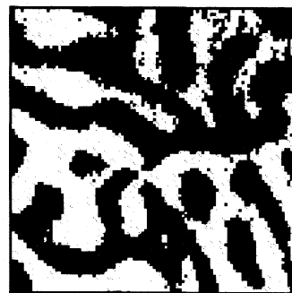
Fig. 9. An example of micro-structure of \text{Al}_2\text{O}_3/\text{YAG} eutectic composite made by image processing (black regions : \text{Al}_2\text{O}_3 single crystal, white regions YAG single crystal).
