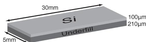
Fig. 9 Si-UF two-layered specimen
